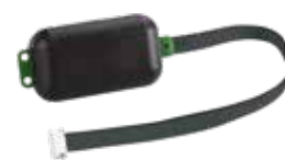
EVIF22TSX TTL/RS-485 serial interface
