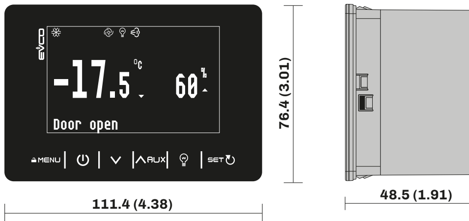
Fig. 1. EVJ 500 series dimensions
