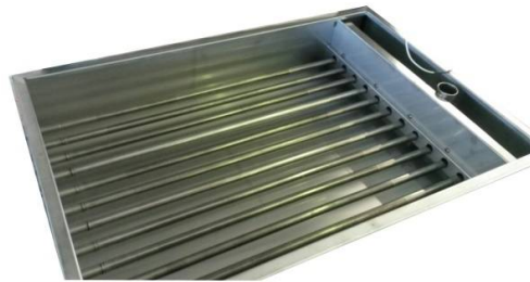
Figura 2 - heaters elements inside kettle
